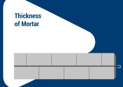
Keep it limited to 10 to 12 mm in cement sand mortar (Refer IS 6041-1985 Para 7, 7.1) & 3 to 4 mm in ready mix mortar.
